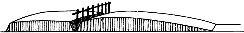
Fig 25 Snow drift on both sides of a fence. on the right completed. on the left incomplete. from a photograph.
